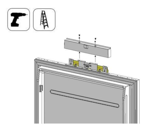
• Loosen 2 screws of the Lower Cover of the Fridge Door and removeit.
