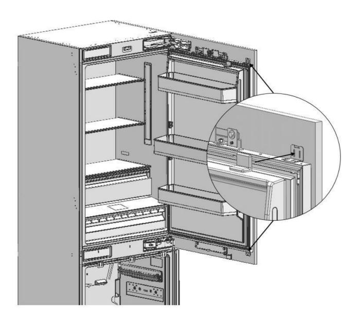
• Use the 4 screws removed from here to fix the upper/lower decoration cover.
