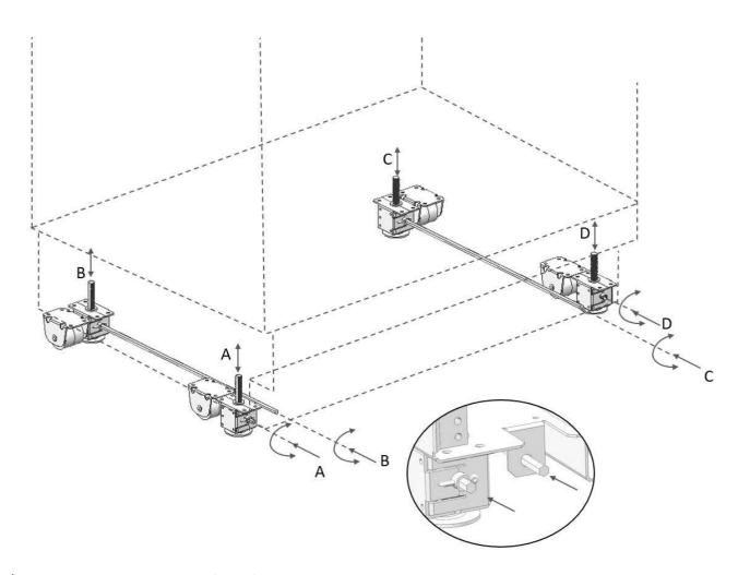
A/D –Turn the key clockwise to lift the front
